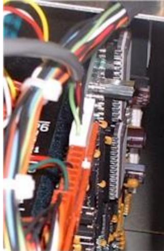
**Figure 7 - HUMAC Serial Cable in P6**
